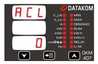
This parameter sets the low limit for low active power alarm.
