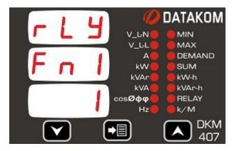
The relay output is a combination of 4 different input functions. The combination logic is explained in the next picture.
