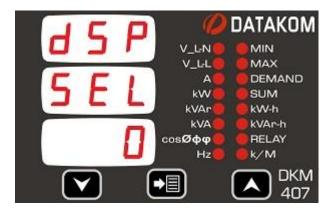
This parameter selects the default screen that the unit returns 5 minutes after any key is pressed.
