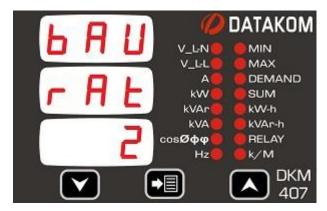
This parameter defines the bit rate used in Modbus communication.
